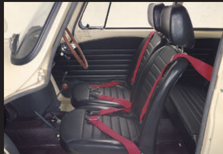
The "Young SS," released in 1968. The front seats were equipped with headrests and three-point seat belts.
