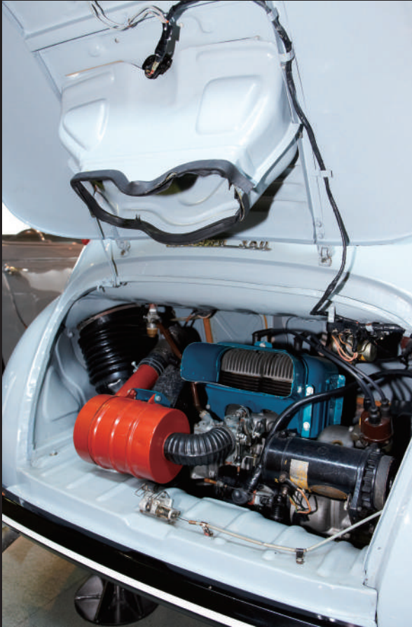
The 2-stroke, 2-cylinder engine mounted at the rear. For forced air cooling, the engine compartment is equipped with ducts to expel cooling air. Air intake to the engine is provided through ducts from the front air cleaner.
