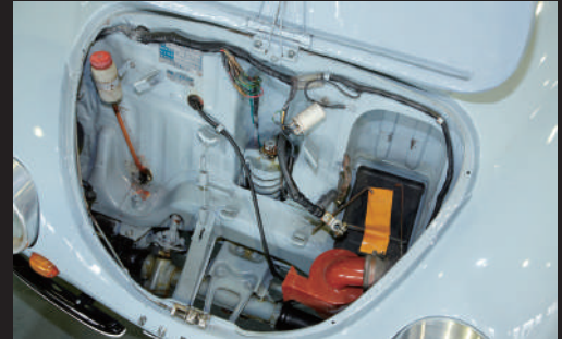
The front hood contains the battery and spare tire and cannot be used as a trunk space.
