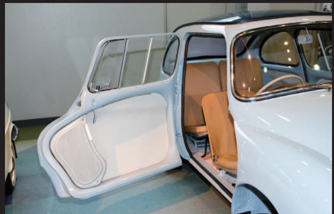
To make it easier to enter and exit the rear seats, the doors are designed with hinges at the rear.
