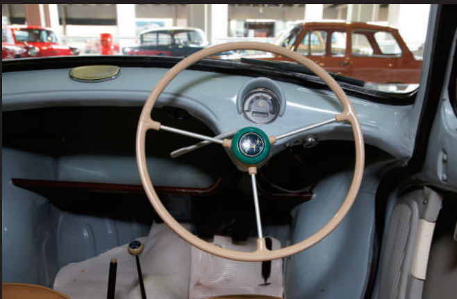
The dashboard area was also simple, with only a speedometer and an odometer as instruments. The controls consisted solely of the steering wheel and a turn signal lever operated with the left hand.
